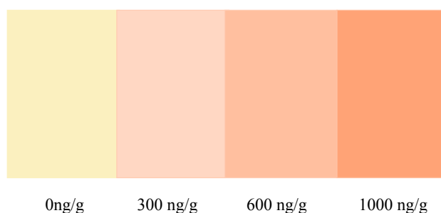
Figure 1: Similar colours to those developed in the detecting papers, using standard solutions equivalent to 0, 300, 600 and 1000 ng/g
